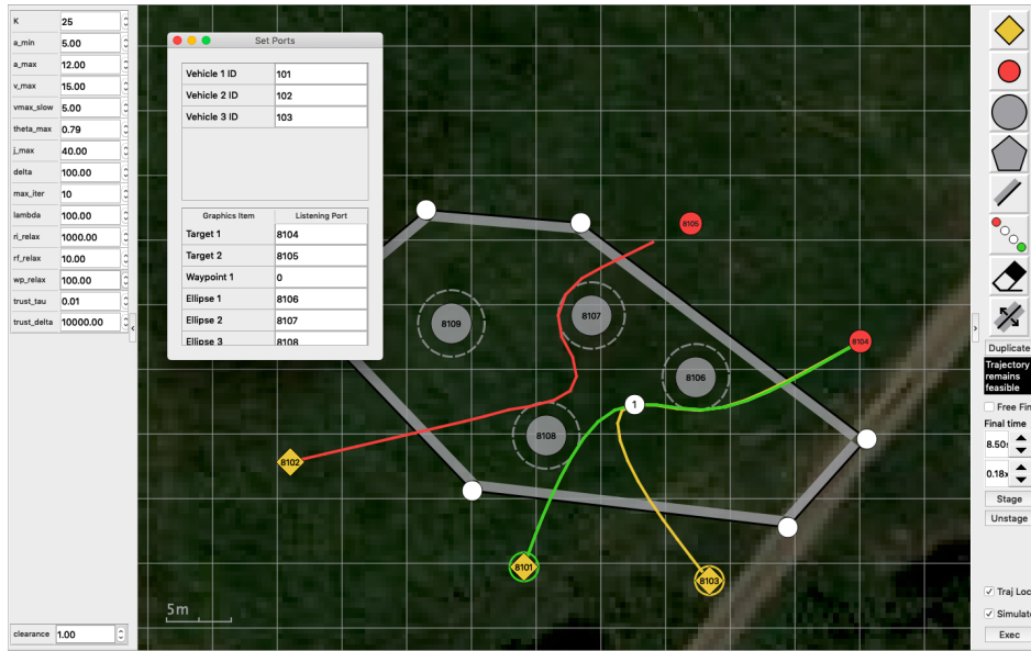
Figure 5: An overview of the visual autonomy interface. Yellow diamonds are the vehicles’ current state, red circles are target destinations, and white numbered circles are waypoints. The gray circles are obstacles and the gray polytope is a slow zone. Each vehicle, target, and obstacle can be tagged to a live tracker using the pop-up window to be updated in real-time. The right panel provides an intuitive interface for non-expert users to update the constraints of the problem, whereas the left panel provides a detailed interface for expert users to fine-tune the optimization algorithms.
