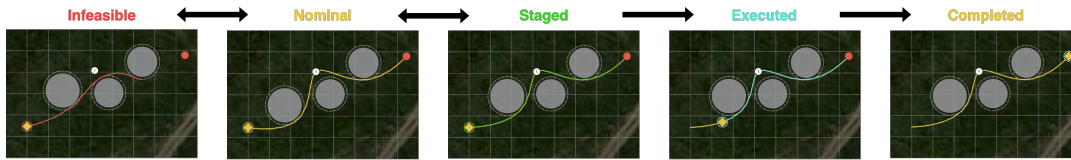
Figure 6: The colors of trajectories represent different stages of execution. Under nominal conditions (yellow), no constraints are violated and the goal can be reached. If the problem is infeasible (red), the users will be alerted on which parameters to adjust to regain feasibility. Once staged (green), the trajectory is locked and is readied for execution (blue). Once completed, it returns to the nominal stage.
