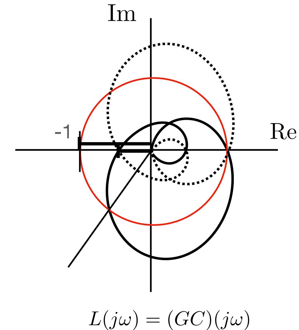
$$\begin{aligned} y &= GC(r - y - n) + d \quad \rightarrow \quad (I + GC)y = GC(r - n) + d \quad \rightarrow \quad y = \underbrace{(I + GC)^{-1}GC(r - n)}_T + \underbrace{(I + GC)^{-1}d}_S \end{aligned}$$
