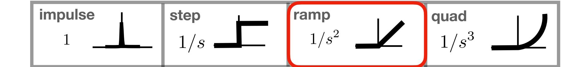
$$\lim_{s \rightarrow 0} \frac{s (s^2 + 2\zeta\omega_n s + \omega_n^2)}{(s^2 + 2\zeta\omega_n s + \omega_n^2) s^2 + 1} \frac{s^2}{K_p s^2 + K_I s + K_{II}} \frac{1}{s^2}$$
