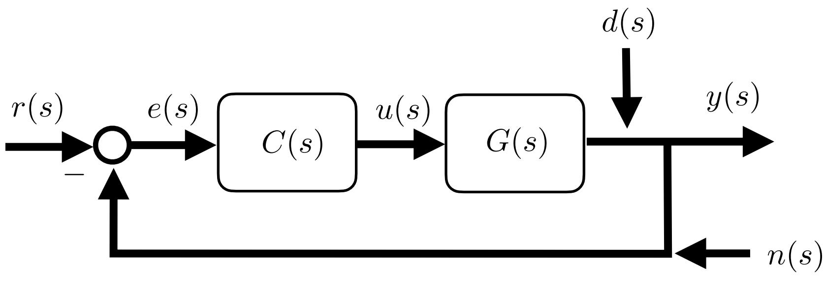
**Loop Transfer**  $L = GC = \frac{n_G}{d_G} \frac{n_C}{d_C}$        $G = \frac{n_G}{d_G}$      $C = \frac{n_C}{d_C}$
