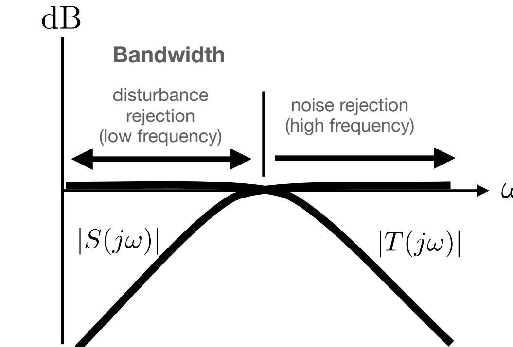
$$\frac{1}{1 + GC} = \frac{1}{1 + \frac{n_G n_C}{d_G d_C}} = \frac{\cancel{d_G d_C}}{\underbrace{d_G d_C + n_G n_C}_{\text{char poly}}} \xrightarrow{\text{given}}$$
