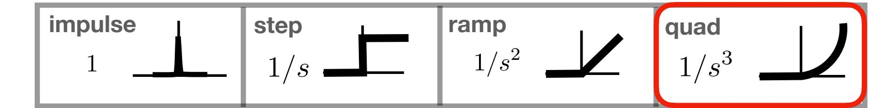
$$\lim_{s \rightarrow 0} \frac{s \frac{(s^2 + 2\zeta\omega_n s + \omega_n^2)}{(s^2 + 2\zeta\omega_n s + \omega_n^2) d_C} d_C}{(s^2 + 2\zeta\omega_n s + \omega_n^2) d_C + 1 n_C} \frac{1}{s^3}$$
