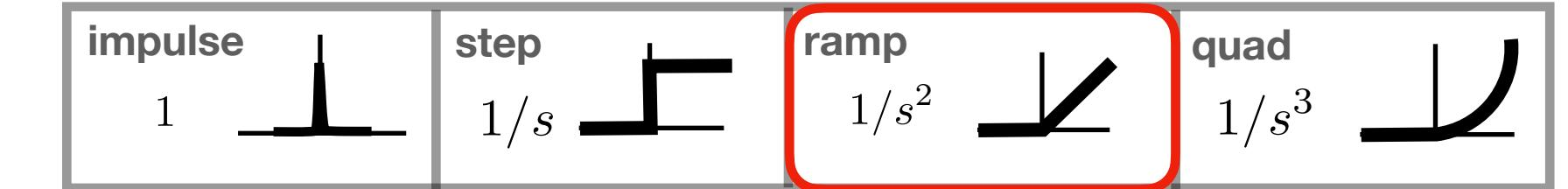
$$\lim_{s \rightarrow 0} \frac{s \frac{(s^2 + 2\zeta\omega_n s + \omega_n^2)}{(s^2 + 2\zeta\omega_n s + \omega_n^2) d_C} d_C}{(s^2 + 2\zeta\omega_n s + \omega_n^2) d_C + 1 n_C} \frac{1}{s^2}$$
