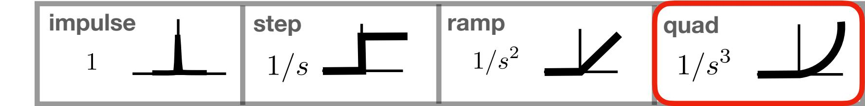
$$\lim_{s \rightarrow 0} \frac{s (s^2 + 2\zeta\omega_n s + \omega_n^2)}{(s^2 + 2\zeta\omega_n s + \omega_n^2)} \frac{s^3}{s^3} + \frac{1}{1} \frac{K_p s^3 + K_I s^2 + K_{II} s + K_{III}}{s^3}$$
