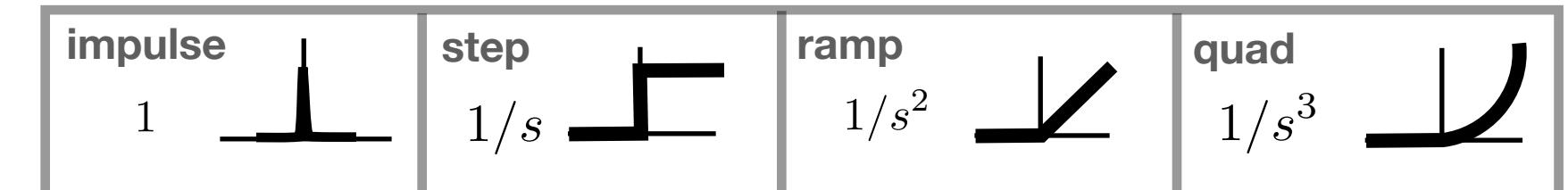
$$\lim_{s \rightarrow 0} sS(s)d(s) = \lim_{s \rightarrow 0} \frac{s \cancel{d_G d_C}}{\underbrace{d_G d_C + n_G n_C}_{\text{char poly}}} \frac{n_d}{d_d}$$
