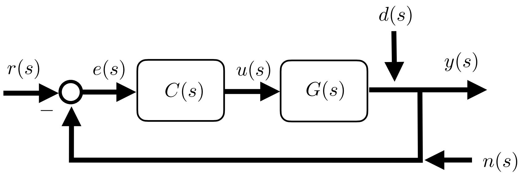
**Loop Transfer**  $L = GC = \frac{n_G}{d_G} \frac{n_C}{d_C}$        $G = \frac{n_G}{d_G}$      $C = \frac{n_C}{d_C}$
