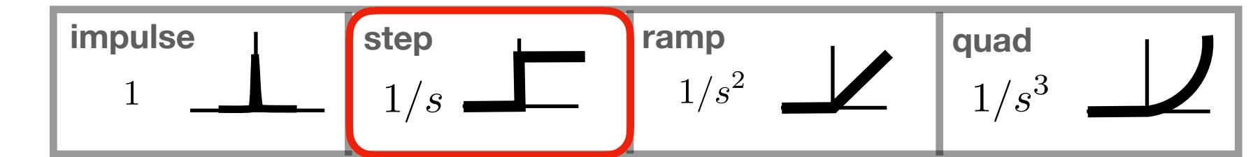
$$\lim_{s \rightarrow 0} \frac{s \frac{(s^2 + 2\zeta\omega_n s + \omega_n^2)}{(s^2 + 2\zeta\omega_n s + \omega_n^2)}}{s + 1 \frac{K_p s + K_I}{s}} \frac{1}{s}$$
