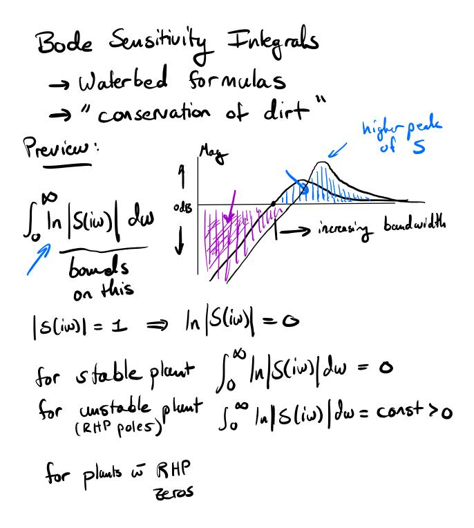
RHP zeros can make the dirt pile up closer to the cross over frequency Second Waterbed Formula: RHP zeros & poles Suppose L(S) has a single, real RHP zero or a conjugate pair of RHP zeros and RHP poles Pk: k=1,..., Np  $\int_{0}^{\infty} \ln |S(iw)| W(z,w) dw = TT \cdot \ln \frac{N_{P}}{TT} |\frac{P_{k}+z}{\overline{P}_{k}-z}|$
