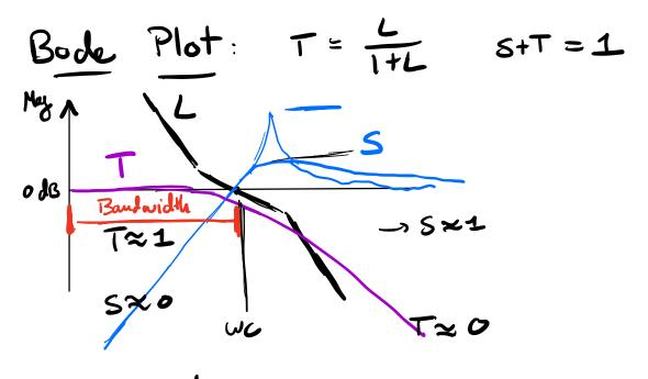
Boundwidth: set of trequencies is good tracking. depends crossover frequency wc faster system response requires larger bandwidth How big can we make the bandwidth of the controller is /out screwing up robustness?
