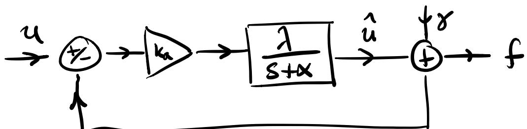
Closed loop feedback system for the thruster w/ a proportional control
