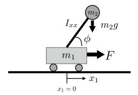
Let m be the mass of the cart,  $I_{xx}$  be the moment of inertia of the pendulum, r the length of the pendulum, and F the force on the cart.
