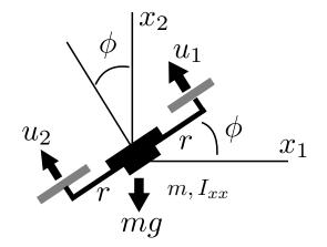
(PTS: 0-6) Given mass m, moment of inertia  $I_{xx}$ , and arm length r, sum the forces and moments to write a nonlinear dynamics model  $\dot{x} = f(x, u)$  for  $x = [x_1 \dot{x}_1 x_2 \dot{x}_2 \phi \dot{\phi}]^T \in \mathbb{R}^6$  and  $u = [u_1 u_2]^T$ .
