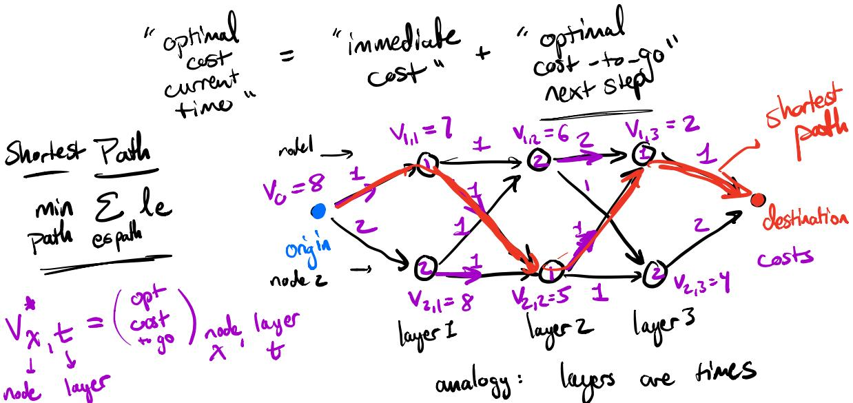
$$V_{1,2} = \min \left\{ \frac{z+z+\frac{V_{1,3}}{2}}{2}, z+1+\frac{V_{2,3}}{4} \right\}$$
